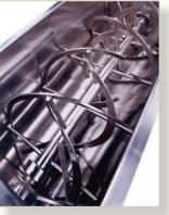
provide a convenient way of controlling speeds during blending and discharging. For most ribbon blender applications, gearmotor/ VFD technology is the most reliable and cost-effective option. Sophisticated PLC systems can be integrated to program steps and recipes in more complex processes.
