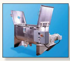
life and eliminates maintenance required to align and adjust belts and couplings. Today's compact gearmotor designs also enable smaller mounting platforms, which improve the ribbon blender's overall space requirement.
